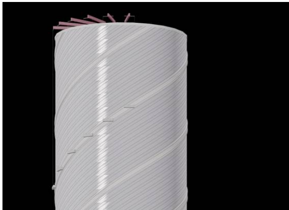
Sketch 1-1 Platform Follows Twist Utilizing Twisting Mullion Tracks and Boom Rotation
