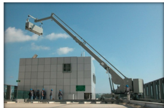
Photograph 5-5 Luffing Boom Allows Cleaning Penthouse and Parapet
