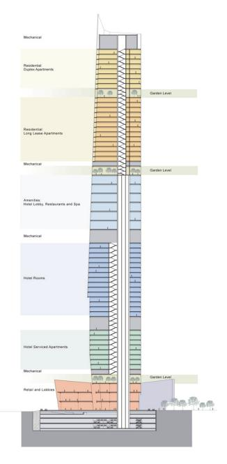
Figure 5: Section Diagram for India Tower, designed by FXFOWLE
