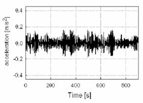
Figure 18. Top Floor Acceleration of the Building with a Passive TLCD
