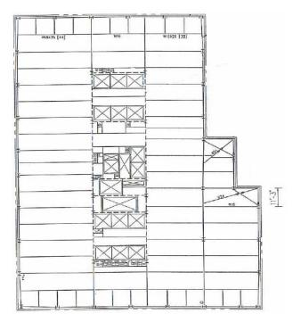
Figure 19. Typical Steel Framing of Random House
