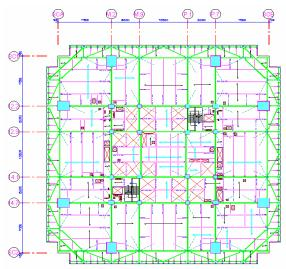
Figure 2. Level 50 Tower Framing Plan of Taipei 101
