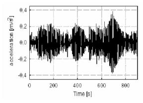
Figure 16. Top Floor Acceleration of the Original Building
