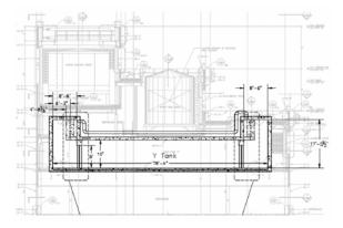
Figure 14. North-South Section through Building Top of Random House
