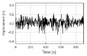
Figure 17. Top Floor Displacement of the Building with a Passive TLCD
