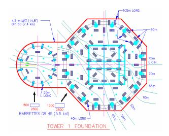
Figure 7. Tower 1 Foundation of One of the Petronas Twin Towers
