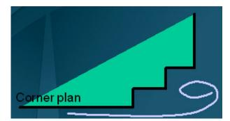
Figure 5: "Saw-tooth corners" used in the wind tests for Taipei 101
