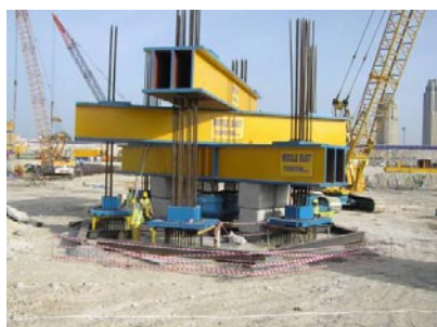
Figure 12 – Test Pile (6,000 tonnes)
