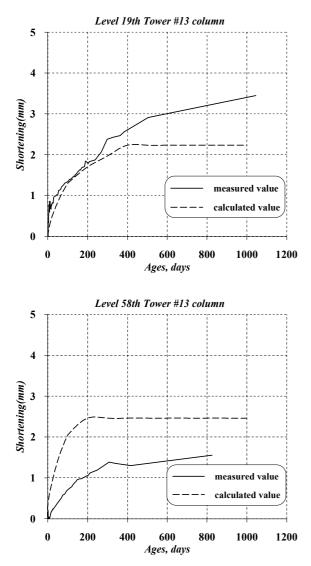
Fig. 2. Measured and calculated values
