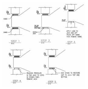
Fig. 15. Sequential Adjustment Steps
