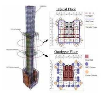
Fig. 2. Framing Plan of Tower
