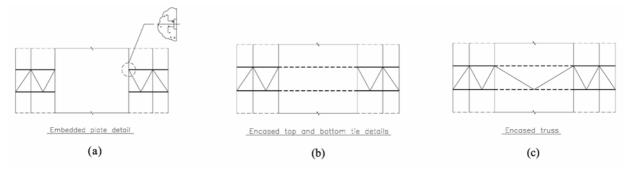
Fig. 13. Connection between Outrigger and Shear Wall
