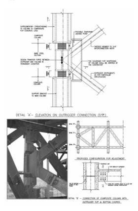
Fig. 14. Connection Details for Outrigger Adjustment
