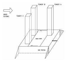
Fig. 7. Transmission of Beam Strip Forces to the Retaining Wall and Soil
