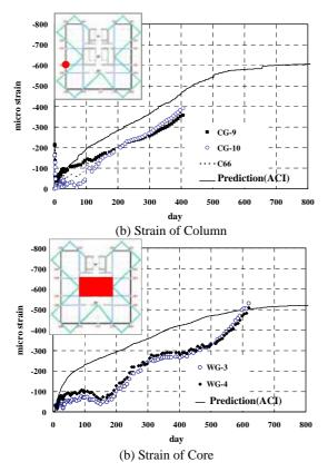
Fig. 12. Axial strain (Prediction & Measurement)
