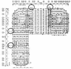
Fig.5. Movement Joint Locations
