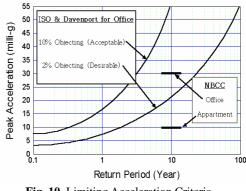
Fig. 10. Limiting Acceleration Criteria
