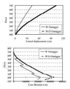
Fig. 8. Effect of the Outrigger
