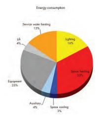
Figure 3. Distribution of energy consumption in Plot 15. (Source: Werner Sobek, Stuttgart)
