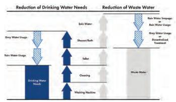
Figure 2. Reduction of water consumption in Plot 15. (Source: Werner Sobek, Stuttgart) 图2. Plot 15减少的用水量 (来源: Werner Sobek, Stuttgart)
