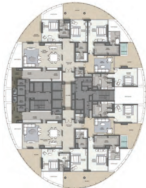
Figure 8. Four Seasons, Delhi: Floor plan of oval of terraces and screens. (Source: Woods Bagot) 图8 新德里四季酒店: 椭圆露台与幕墙的平面图 (来源: 伍兹贝格)
