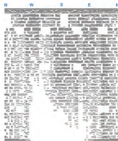
Figure 9. Four Seasons, Delhi: Unfolded elevation mapping screen panel types. (Source: Woods Bagot) 图9 新德里四季酒店: 立面幕墙面板类型展开图 (来源: 伍兹贝格)
