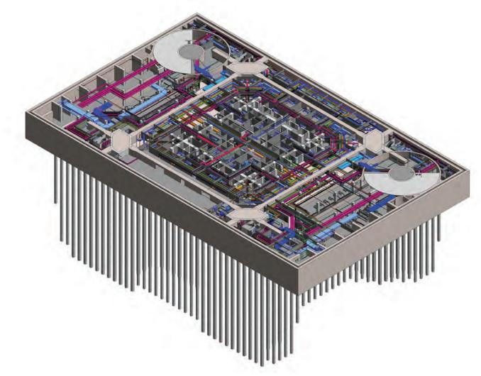
Figure 5. China Zun MEP technicial room study (Source: Beijing Institute of Architectural Design) 图5. 中国尊地库层机电综合空间研究 (出自: BIAD)
