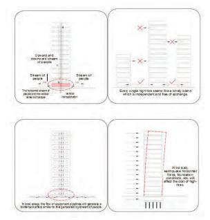
Figure 1. The challenges of high-rise buildings 图1.高层建筑面临的挑战
