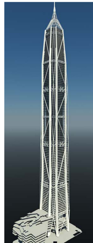
Figures 16(left), 17(top), 18(bottom), 19(right). Ping An rendering showing notched corners, core and outrigger arrangement, belt truss, and mirrored bracing pattern. Credits: KPF, all others Thornton Tomasetti.
