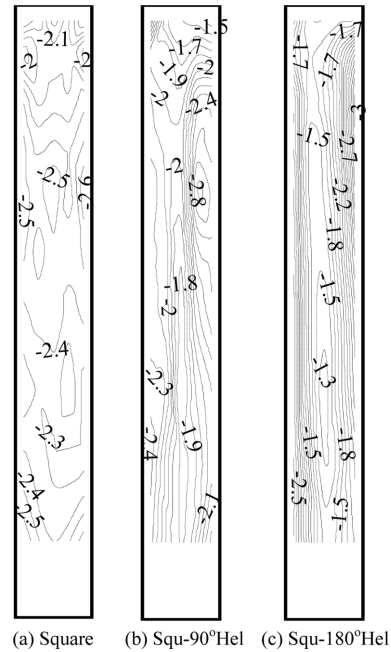
Figure 17. Largest negative peak pressure coefficients for all wind directions for Square helical models.
