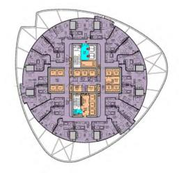
Figure 4.10. Arrangement of Stairs in Zone 7 (Source: Gensler, 2009) 图4.10. 区域7内楼梯布局(来源: Gensler, 2009)
