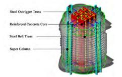
Figure 4.5. Tower Structure (Source: Gensler, 2009) 图4.5. 大厦结构 (来源: Gensler, 2009)
