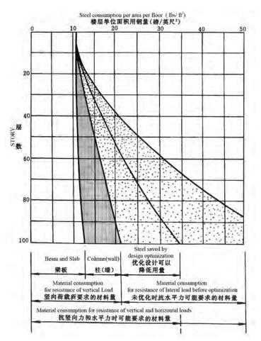
Figure 3.48. The change of structural cost with structural height (Source: Lin T.Y. & Stotesbury, S.D.) 图3.48. 结构成本随结构高度的变化 (来源: 林同炎 & Stotesbury, S.D.)
