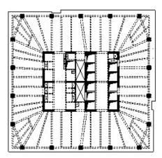
Figure 3.49. Floor systems layout optimization – Optimization design scheme (Source: Xin Zhao) 图3.49. 楼盖体系布置优化案例 – 优化设计方案 (来源: 赵昕)
