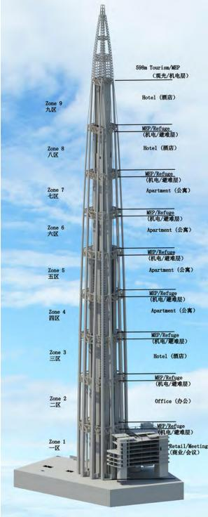
Figure 3.47. Tower Main Lateral System (Source: Thornton Tomasetti) 图3.47. 塔楼主体抗侧力体系 (来源: 宋腾添玛沙帝)
