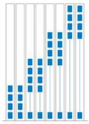
Zoned groups with elevators using carbon-fiber rope, split between low rise, mid rise, high rise, and ultra-high rise.
