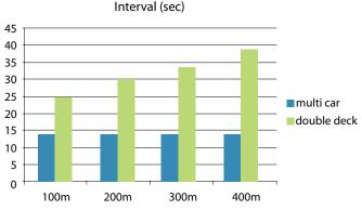
Graph 6: Comparison of multicar vs. double deck depending on travel height: interval. Source: ThyssenKrupp
