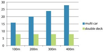
Graph 5: Comparison of multicar vs. double deck depending on travel height: number of cabins. Source: ThyssenKrupp
