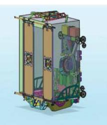
Opposite: A circulating rope-less elevator system called MULTI. Source: ThyssenKrupp
