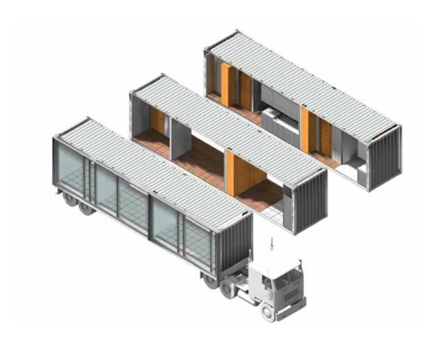
with the eight steel corner nodes which enable automated intermodal handling. We'll call that new type of building module a Volumetric Unit of Construction, or VUC, to clearly distinguish it from a shipping container.
