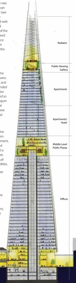
Figure 4. Section drawing of The Shard (Source: Renzo Piano Building Workshop)
