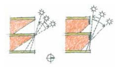
Figure 2. Sketch section. Subtropical conditions call for flexible and adaptable measures such as shading devices to account for welcoming the sun deeper in winter (left) or excluding sun in summer (right) (Source: Centre for Subtropical Design)
