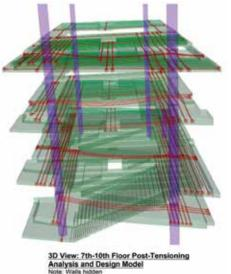
Figure 8. Bonded post-tensioning system as idealized during structural analysis and as constructed (Source: Columbia University Left / Leslie E. Robertson Associates)
