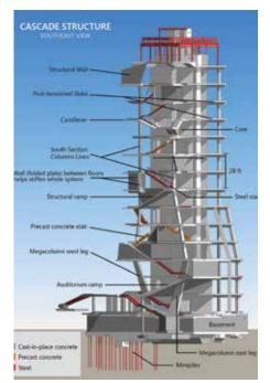
Figure 11. Overview of the structural components of the Cascade (Source: Leslie E. Robertson Associates)
