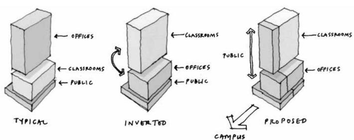
Figure 2. Building massing diagram identifying the vertical arrangement of public space on the campus-facing south façade, defining the "Study Cascade". (Source: Diller Scofidio + Renfro)
