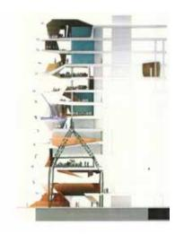
Figure 12. Competition-phase visual narrative that identifies the fundamental framework of the Cascade's structure and sets the stage for systems development in future phases (Source: Leslie E. Robertson Associates)
