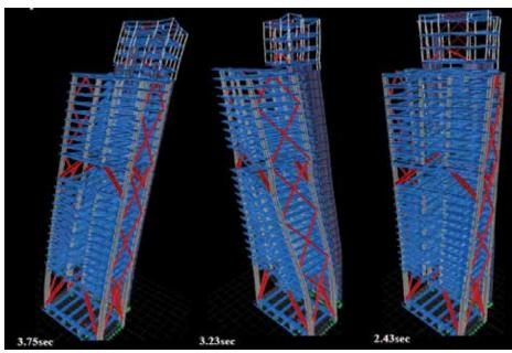
Figure 9. Fundamental dynamic mode shapes (Source: Arup)
