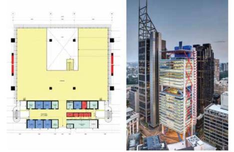
Figure 1. Typical village floor plan at architectural concept, and completed building. Only two columns are located within the floorplate on the village floors (Source: RSHP & Brett Boardman)
