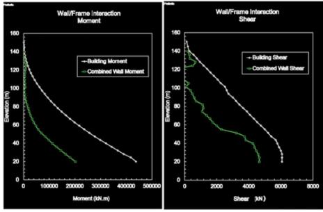
Figure 4. Distribution of moment and shear between the cores and braced frames under wind loading in the northsouth direction (Source: Arup)
