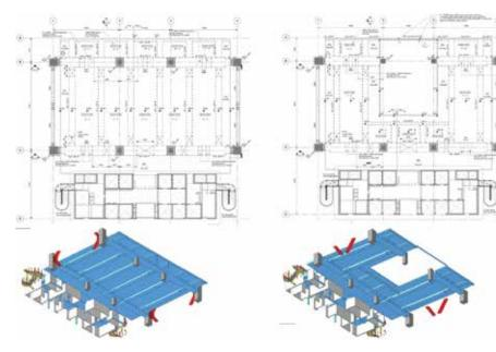
Figure 3. Typical floor structure. Full floor (left) and village floor (right). 3D views from below under (Source: Arup)
