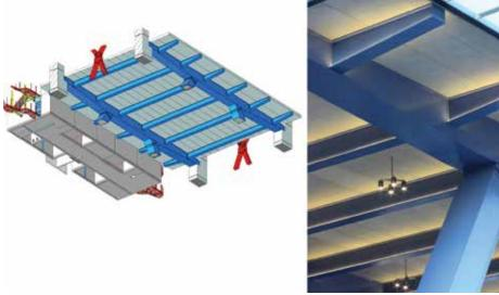
Figure 8. Reverse podium structural arrangement and completed structure (Source: Arup)
