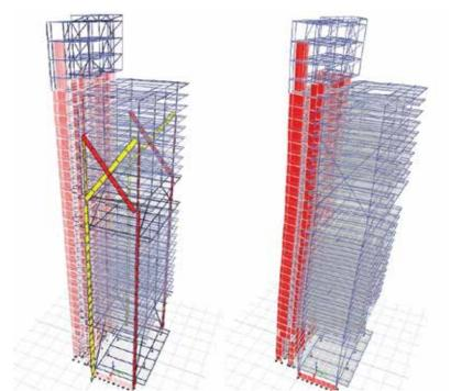
Figure 6. Structural analysis under fire load case with Zone 2 fire condition (Source: Arup)
