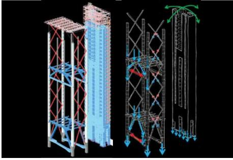
Figure 2. Stability and Gravity System (Source: Arup)
