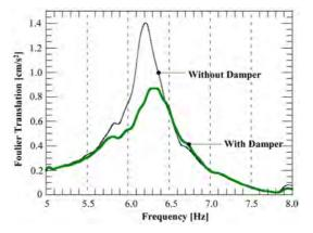
Figure 12. Measurement of floor vibration.
