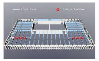
Figure 11. Damper Location on typical floor.
