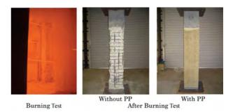
Figure 16. Fire Resistance Experiment.
