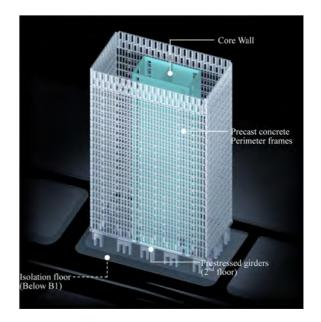
Figure 2. Structural perspective.
