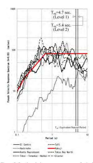
Figure 7. Pseudo velocity response spectrum of seismic waves in design.
