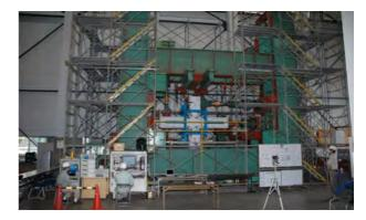
Figure 15. Beam-Column Joint Experiment.
