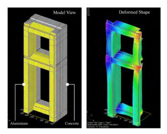
Figure 13. Thermal stress analysis.
