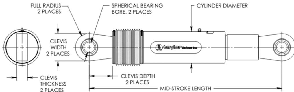
**Figure 5.** Taylor device geometric and mechanical properties.
