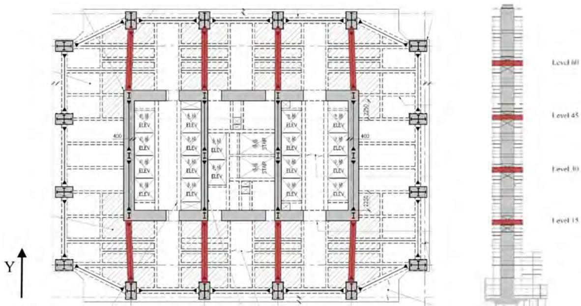
**Figure 7.** Typical outrigger floor and section of the example structure (position of the outriggers/dampers shown in red).
