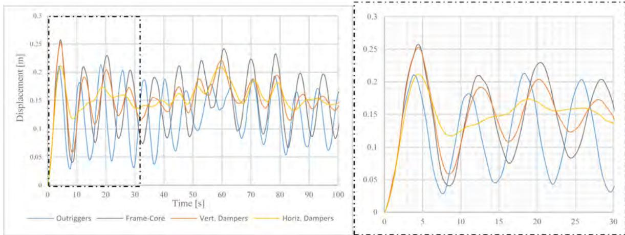
**Figure 15.** Displacement history for 50-year return period Wind load case. Full history (left) and enlargement (right).
