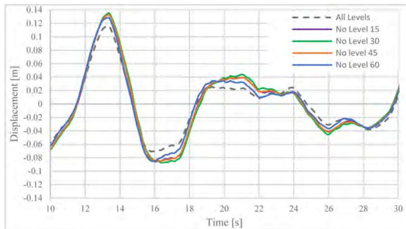
**Figure 20.** Roof displacement response under Frequent Earthquake of several configurations of horizontal dampers.
