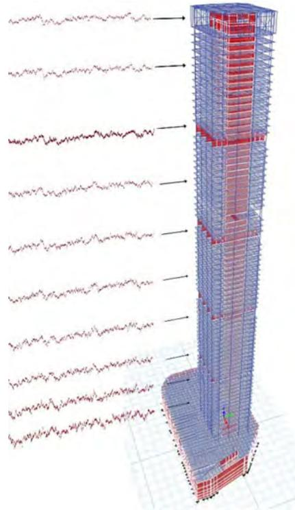
**Figure 9.** Wind loads as applied on the model.
