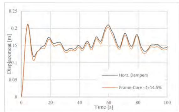
**Figure 19.** Displacement response comparison for computed damping ratio validation (horizontal dampers) - 50-year Wind.
