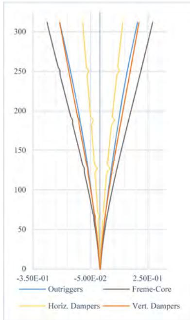
**Figure 12.** Story displacement results for Frequent Earthquake load case.
