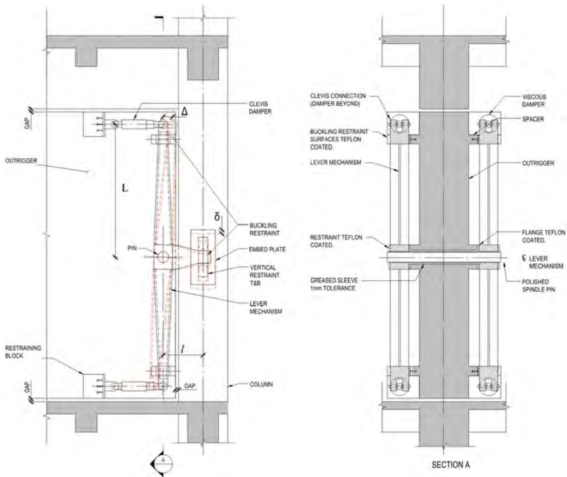
**Figure 2.** Schematic components the amplification mechanism (displaced configuration of the system shown in red).
