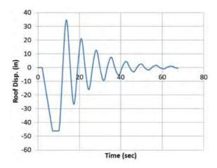
Figure 3. decay of deflection caused by damping.
