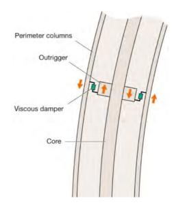
**Figure 1.** the damped outrigger concept (Image copyright Arup).
