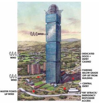
Figure 6. Allocating the muster points © Yas Architecture
