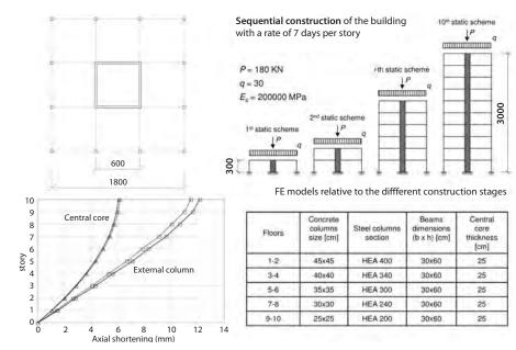
Figure 4. ASAP software validation – case study relative to a multistory building with concrete core and concrete or steel columns (sequential construction). Layout plan, analysis models relative to the different construction stages. Axial shortening is shown, corresponding to different floors at 100 years (concrete structure) and to the characteristics of the structural members adopted in the comparison.
