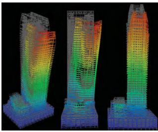
Figure 7. Deformed shape of the Public Mutual Tower at target time of 100 years.
