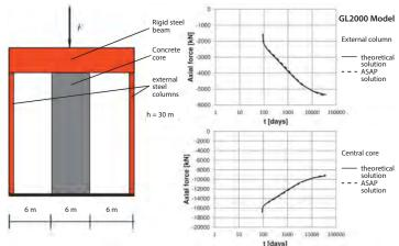
Figure 3. ASAP software validation - case study relative to a non-homogeneous hybrid
