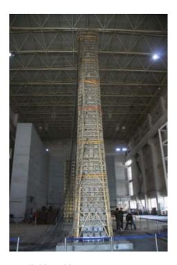
Figure 15. Shaking table test.
