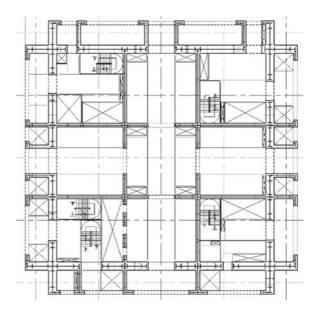
Figure 8. The core plan at lower floors.
