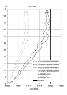
Figure 9. Inter-story drift by earthquake and wind.
