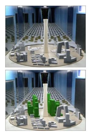
Figure 11. Different proximity scenarios in wind tunnel tests (© RWDI).
