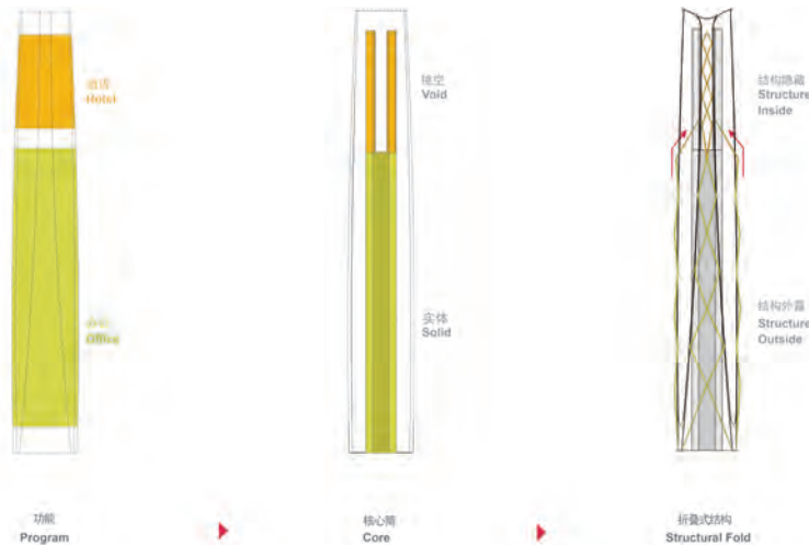
Figure 10. The shift in the structural system occurs at the boundary between the tower's two functions (Source: HENN)
