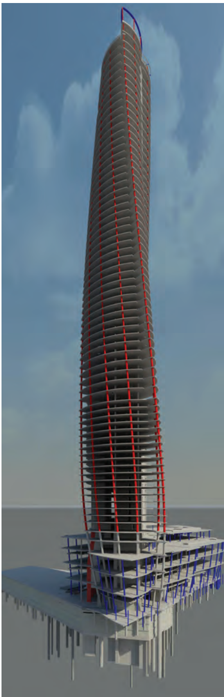
Figure 6. 3-D view of the tower (Source: Robert Bird Group) 图6. 结构地上主体和地下结构分析3维模型 (来源: Robert Bird Group)
