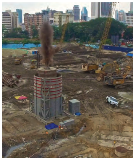
Figure 1. Statnamic load test (Source: PMV) 图1. 静载试验 (来源: PMV)
