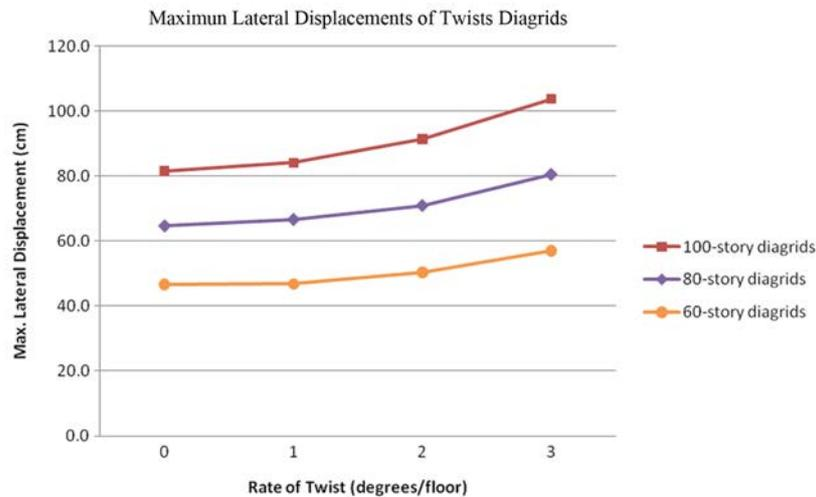
**Figure 4.** Maximum lateral displacements of twisted diagrids of various heights.
