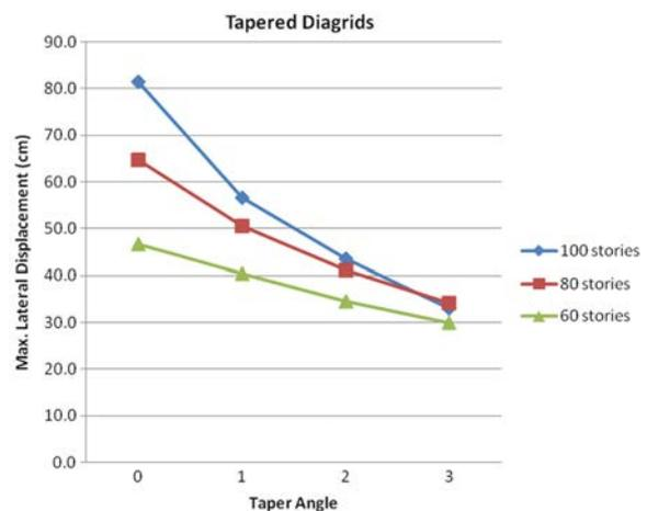
**Figure 10.** Maximum lateral displacements of 60-, 80- and 100-story tapered diagrids.
