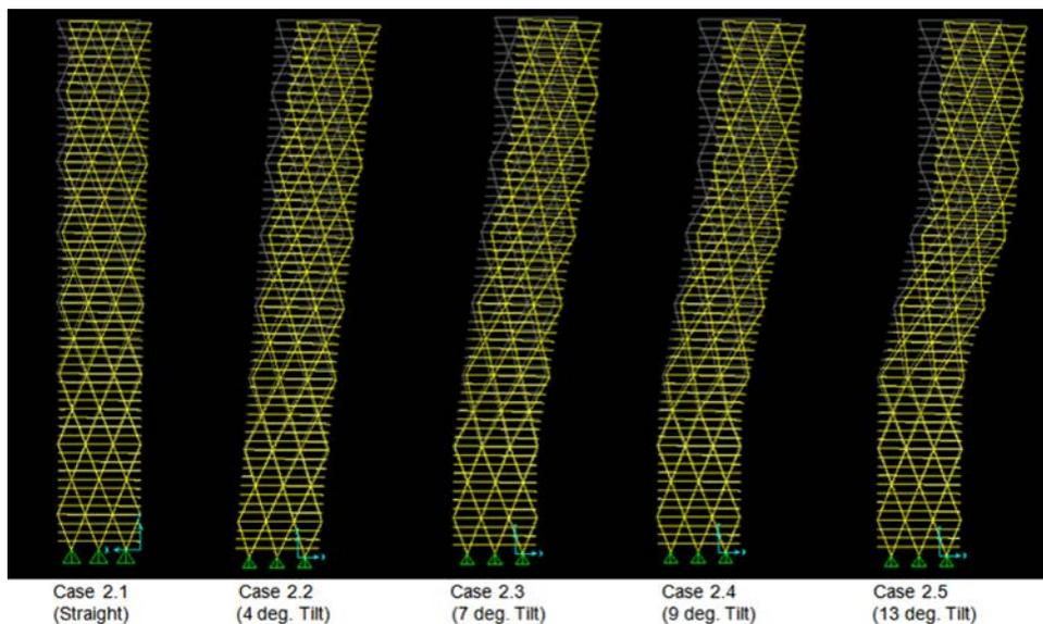
**Figure 6.** 60-story tilted diagrid structures with tilted angles of 0, 4, 7, 9 and 13 degrees.
