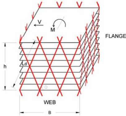
**Figure 1.** An 8-story diagrid module.
