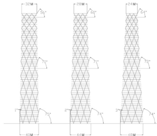
**Figure 9.** 60-story tapered diagrids design Alt.2: diagrid members are placed at angles steeper toward the base.
