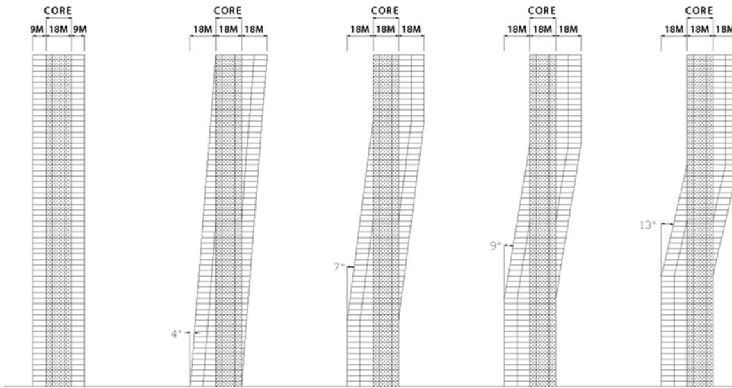
**Figure 5.** 60-story tilted diagrid structures with tilted angles of 0, 4, 7, 9 and 13 degrees (section view).
