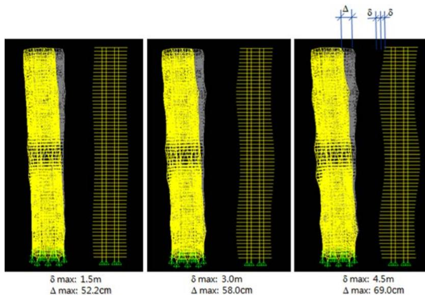
**Figure 11.** 60-story freeform diagrids' deformed shape in 3D (left), undeformed section through core in 2D (right).
