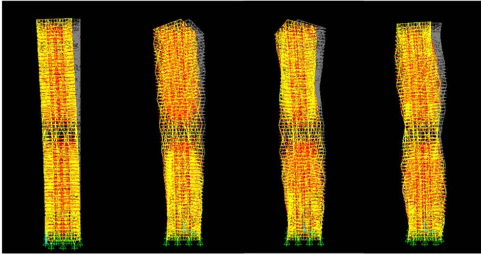
**Figure 3.** 60-story diagrids structures of various rates of twist.
