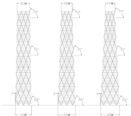
**Figure 8.** 60-story tapered diagrids design Alt.1: diagrid members are placed at angles steeper toward the top.
