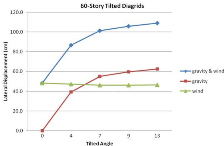
Figure 7. Maximum lateral displacements of the tilted diagrid structures shown in Fig. 6.
