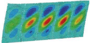
Figure 9. SPSW pushover model and deformed shape
