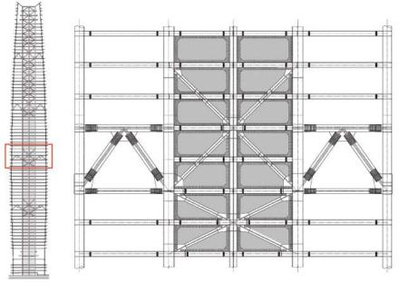
Figure 4. Outrigger truss
