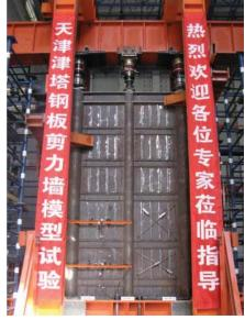
Figure 10. SPSW assembly test set-up
