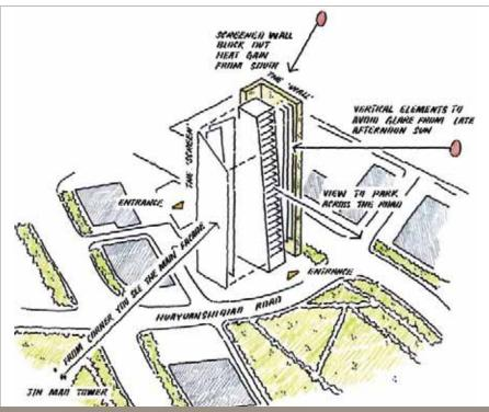
Figure 8. Different solar and amenity requirements governed the cladding design on each elevation of the BEA Tower in Shanghai (TFP Farrells)
