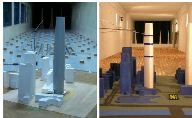
**Figure 31.** HFBB wind tunnel test.
