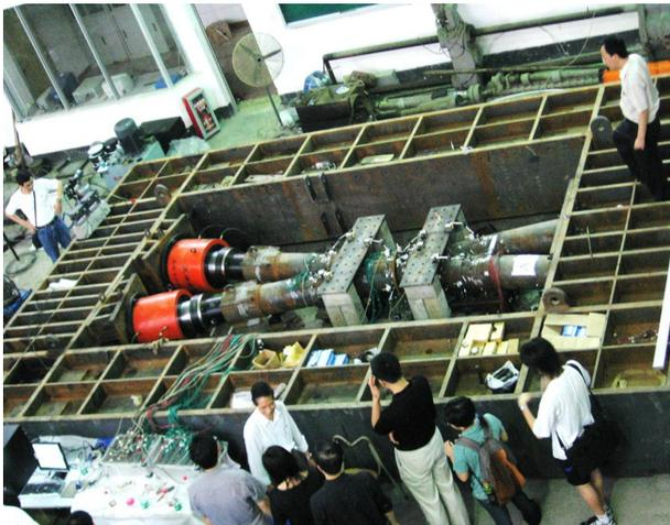
**Figure 41.** Large-scale testing of nodal connection.
