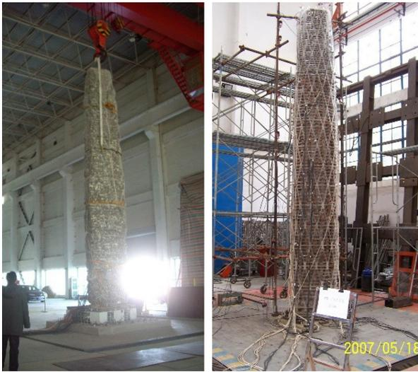
**Figure 37.** Shaking table test.
