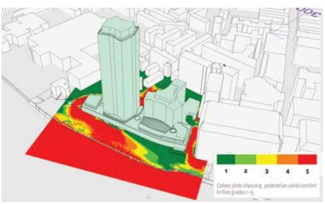
Figure 11. Year-round pedestrian wind comfort visualization on a horizontal plane at 1.5 m above grade, according to Dutch Wind Nuisance Criteria, for the Millbank Tower.
