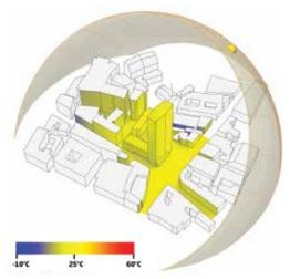
Figure 8. Simulated surface temperatures as a result of the full thermal energy balance simulation on the Centre Point Tower façades and surroundings on April 29,1:00 p.m.
