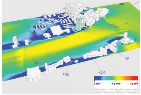
Figure 10. Results of the CFD simulation visualizing wind velocities on a horizontal plane at 1.5 m above grade for the 30° heading (NNE) for the Millbank Tower in London.
