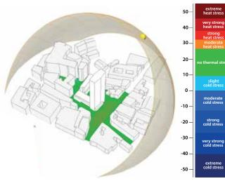
Figure 9. Simulated UTCI Equivalent Temperature on a horizontal plane at 1.5 m above grade for the area around Centre Point Tower on April 29, 1:00 p.m.
