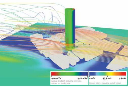
Figure 12. Results of the CFD simulation visualizing façade pressure values on the South Bank Tower.
