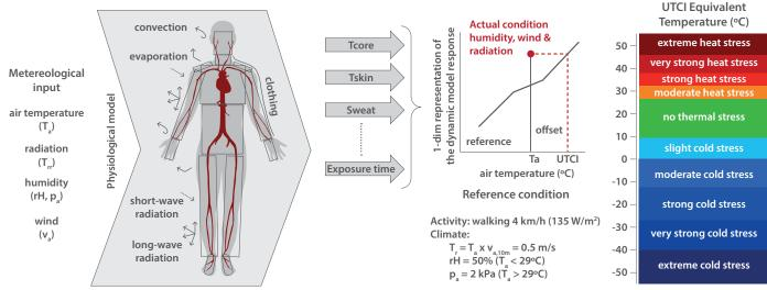
Figure 4. The Universal Thermal Comfort Index (UTCI) Equivalent Temperature identifies comfort in an urban space via a relative temperature scale.
