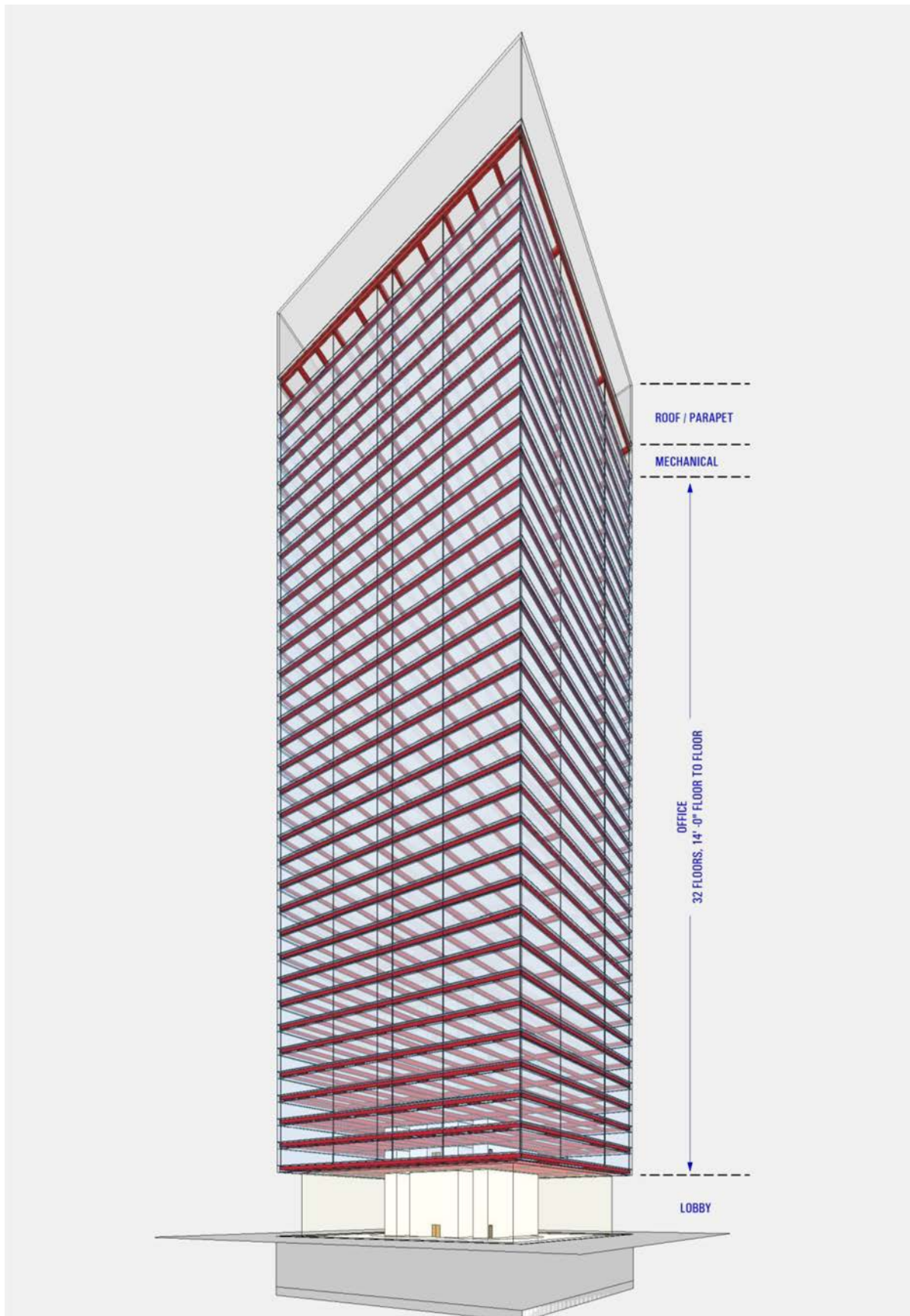
Figure 10. Diagram of 550' Office Tower using Core Cantilever Construction.
