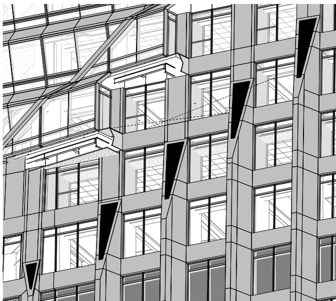
Figure 6. The accordion-shaped exterior wall of Akhmat Tower, designed in Revit with 12 control points per panel.
