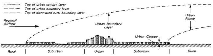
Figure 1. Schematic representation of the urban atmosphere, illustrating proposed two-layer Canopy and Boundary Layers classification. Source: Oke, 1976
