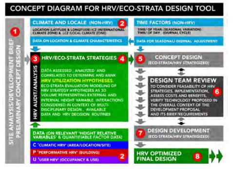
Figure 8. Concept diagram for HRV/eco-strata design tool.
