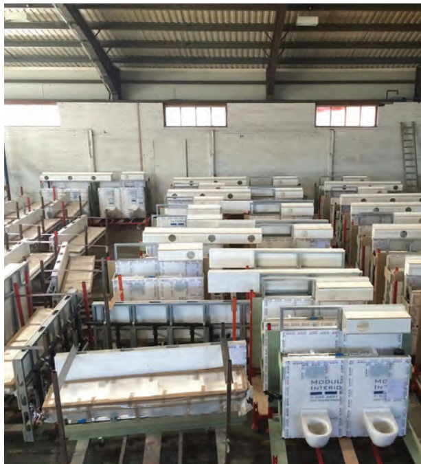
Figure 10. Large scale pre-fabrication of bathrooms units (left) developed by Modular Interiors for the construction of 100 Bishopsgate, London (right). © Allies & Morrison and Arney Fender Katsalidis
