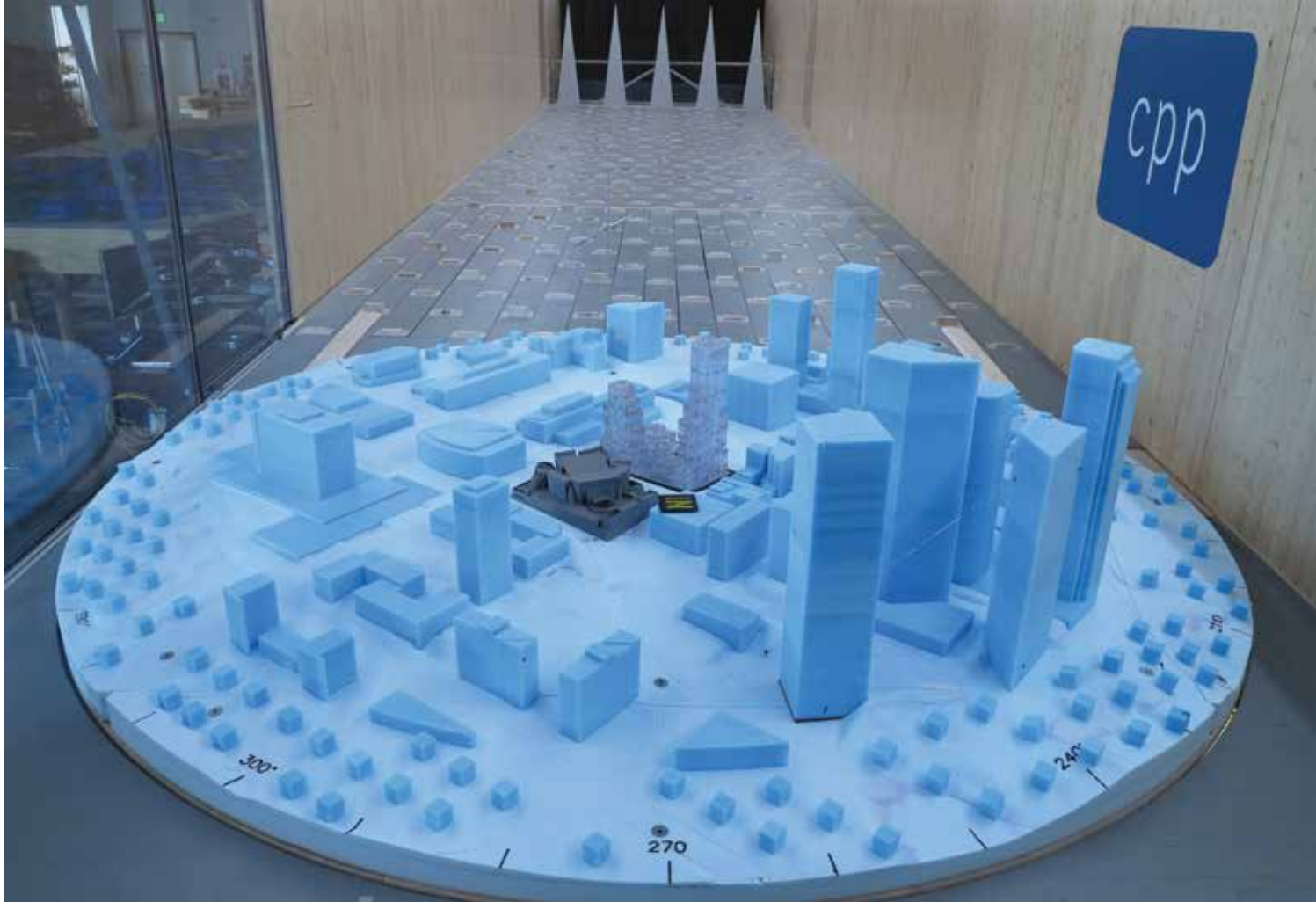
Figure 2. Typical boundary layer wind tunnel test showing pressure test and proximity models on turntable and boundary layer generation devices including trip board, spires, and floor roughness. © CPP Wind Engineering
