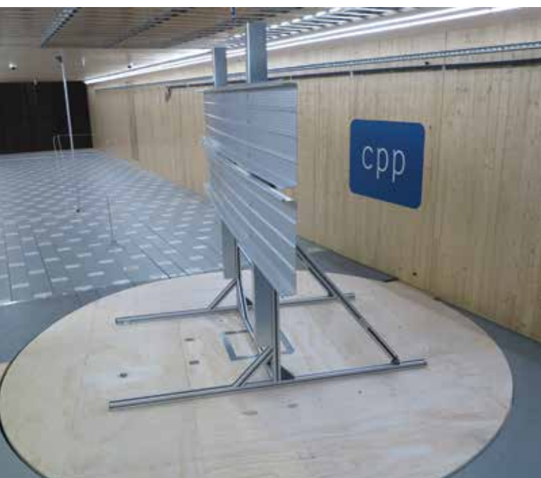
Figure 4. Sample of porous cladding being tested for noise in the wind tunnel. © CPP Wind Engineering
