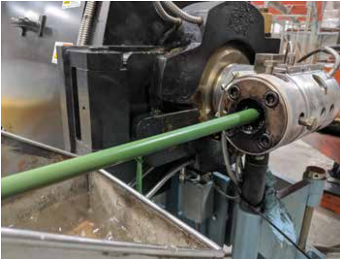
Figure 1. Plastic extrusion process. © Neel Khosa
