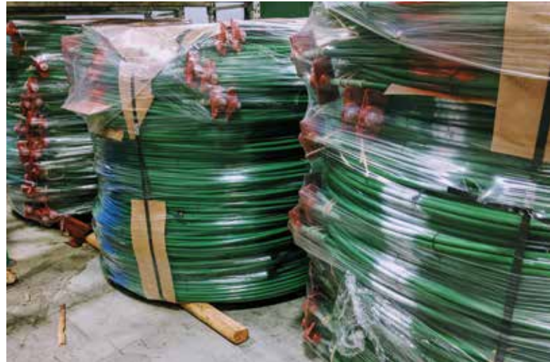
Figure 2. Unbonded PT bundle of tendons. © Neel Khosa
