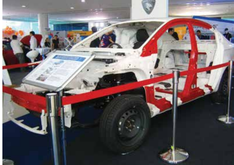
Figure 4. The integration of the frame and body into a “unibody” was one significant move that made cars lighter, stronger and faster to build. © Aero7 (cc by-sa)
