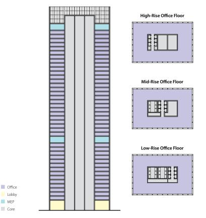
Figure 3. Section drawing and plans of the sample generic building used for the research. There are 18 passenger-rated elevators in three banks, serving floors 1–15, 16–28, 29–43, respectively. MEP floors are located at floors 15 and 43. © CTBUH
