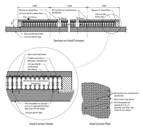
Figure 4. Placement of the ecobricks was determined after numerous iterations. The bricks form voids that would normally be occupied by EPS or lightweight concrete. © Arup
