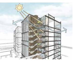
Figure 5. Recesses cut out along building elevations allow sunlight and ventilation to enter the buildings.
