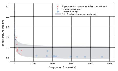
Figure 10. Graph illustrating the discrepancy between the available timber compartment fire tests and the proposed or constructed high-rise mass timber buildings.
