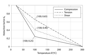
Figure 5. Reduction in compressive strength parallel to the grain in softwoods, plotted against rise in temperature. Source: BS EN 1995-1-2, 2009
