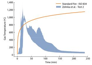
Figure 4. Graph showing the difference between the standard fire (CAN/ ULC S101) and the temperatures from a compartment fire (natural fire curve). Source: Taber et al. 2014
