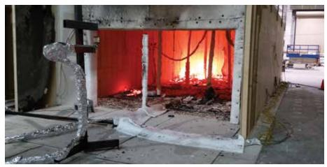
Figure 8. CLT compartment fire from the Fire Protection Research Foundation series of tests.
