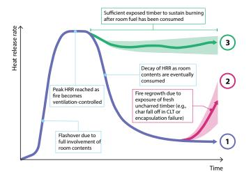
Figure 2. General trend lines of heat release rate (HRR) vs. time plots from experimental data of ventilation-controlled fires within exposed CLT compartments.
