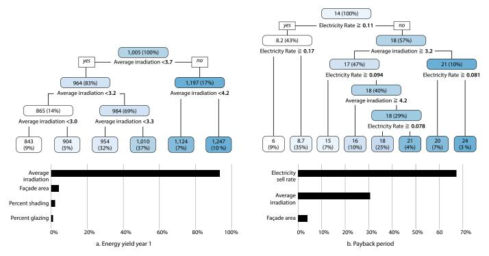
Figure 6. Result of classification and regression tree analysis. Model (a), at left, examines the effect of monthly average solar irradiation, façade area, and glazing percentage on energy yield. Model (b), at right, compares the amount of influence irradiation levels, electricity rates, and façade area have on time to payback of an investment in BIPV panels.
