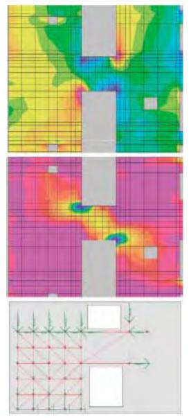
Figure 5. Stress contours adjacent to the opening and the selected strut and tie arrangement
