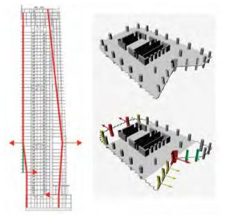
Figure 2. Diagram of unbalanced forces on structural system. 图2. 结构体系不平衡力示意图
