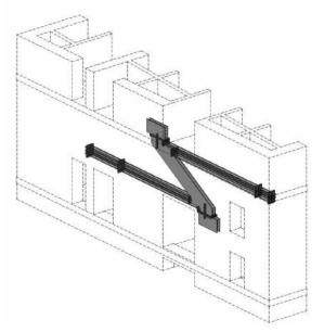
Figure 6. Axonometric view of mega link beam 图6. 巨型连梁轴测图
