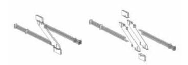
Figure 7. Exploded view of mega link beam showing individual components. 图7. 显示每个单独部件的巨型连梁分解图
