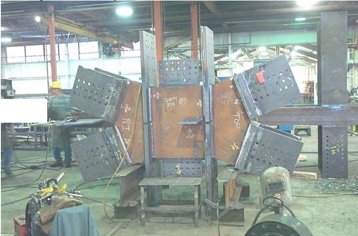
Figure 17- The Diagrid Node after assembly construction for use on the Swiss Re
