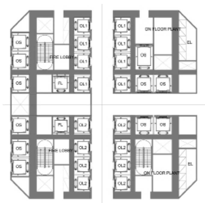
Figure 9. T-shaped-pattern Arrangement of Core Tubes, drawn by Lijie 图9. 丁字形核心筒布局示意（出自：作者自绘）
