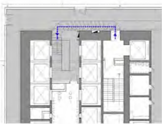
Figure 10. Stair Conversion in the Refuge Floor, the Skyscraper in Commercial Center of Nanshan, Shenzhen
