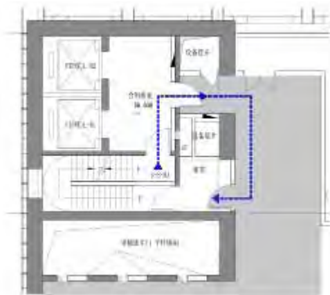
Figure 11. Stair Conversion in the Refuge Floor, Tianchen Tower
